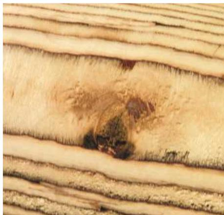
▲ Pic.14 Even though this is top-grade ply there is the likelihood of coming across defects in the wood. These don't seem to detract from the finished lamp base though
